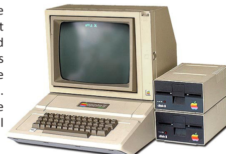
The Apple II was introduced in 1977. An 8-bit computer, it was one of the first mass-produced microcomputers - its success was due primarily to its aggressive marketing to educational institutions. By the end of production in 1993, ~5-6 million Apple IIs were sold.
